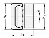
In the combination of rails GN 2422 and cam roller carriages GN 2424, the following dimensions / tolerances exist.
