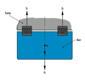
= maximum working radial load of the hinge [Newton] **Ea** = maximum working axial load of the hinge [Newton]
