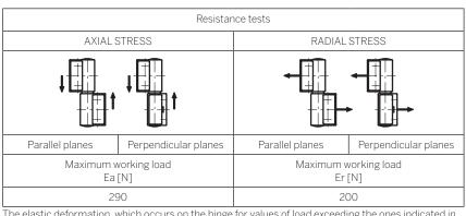
The elastic deformation, which occurs on the hinge for values of load exceeding the ones indicated in the table, makes the load at breakage meaningless.
